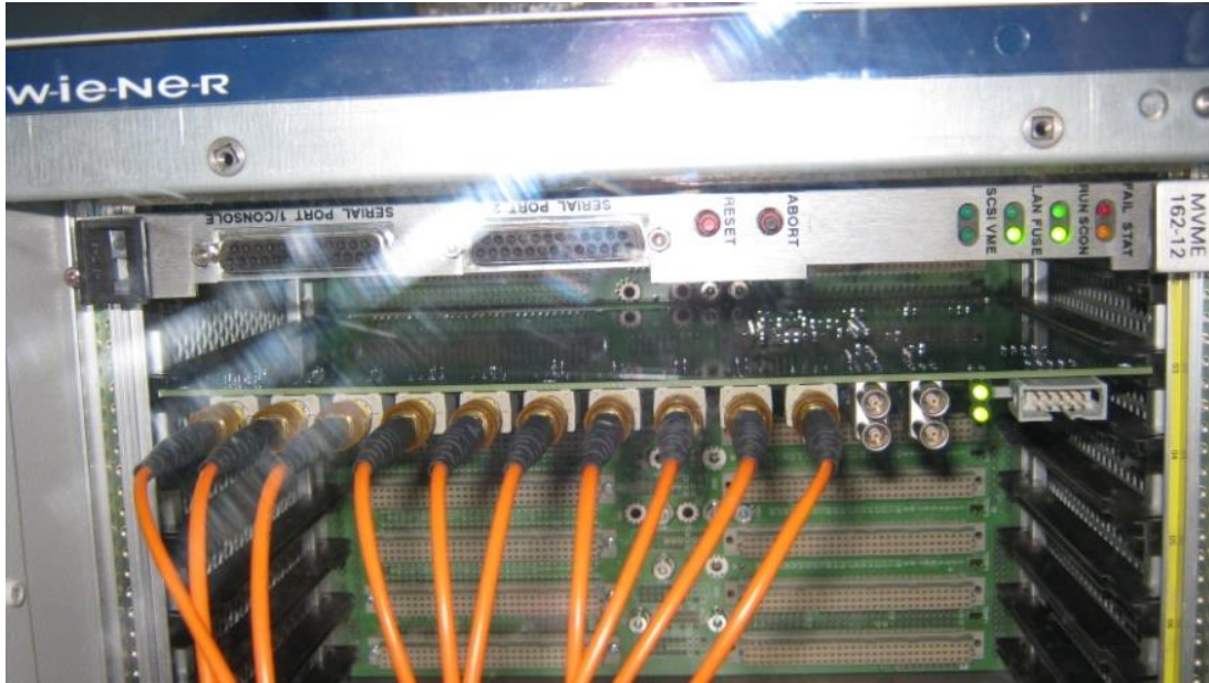
Figure 4: Helicity Control Board and its crate. The name of the crate is “iochelgen”. There are 12 fibers connected to this crate. The first 10 fibers carry signals to (Line Sync) and from (9 signals) the Helicity Board. Fiber 11 is iochelgen TX and Fiber 12 is iochelgen RX.
