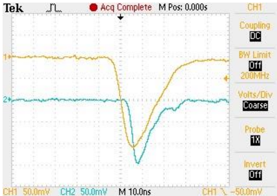
Figure 4: E and DE raw detector signals.
