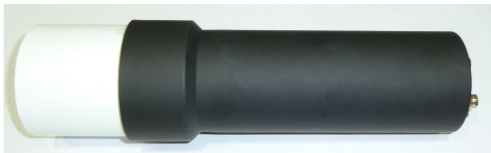
Figure 2: E detector (before wrapping it with black tape).
