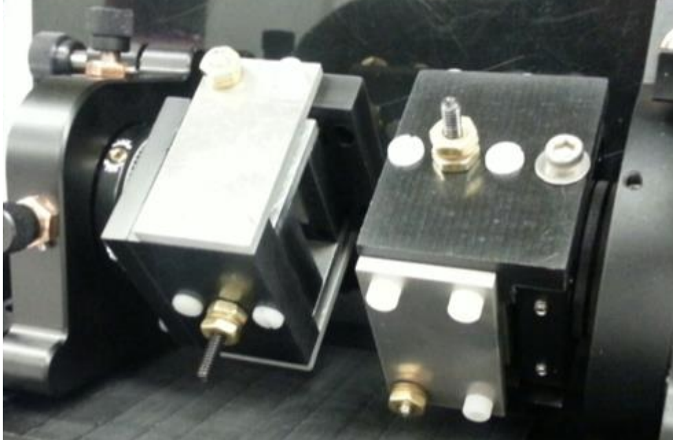
Figure 4: RTP Cell mounting with two crystals.
