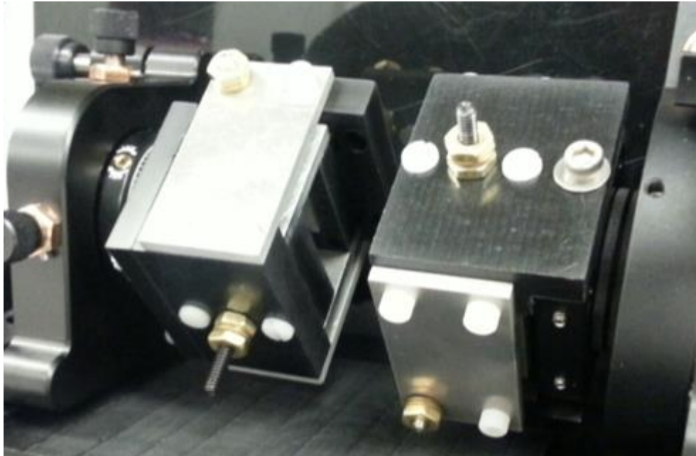
Figure 4: RTP Cell mounting with two crystals.
