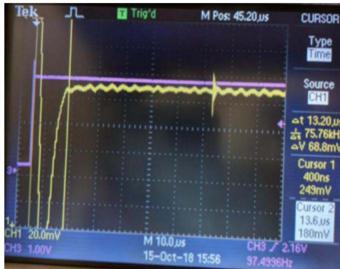
Figure 2: 13 \mu s transition time with <1% ringing.
