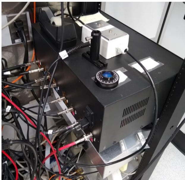
Figure 6: RTP Pockels cell HV supply used at CEBAF laser table.
