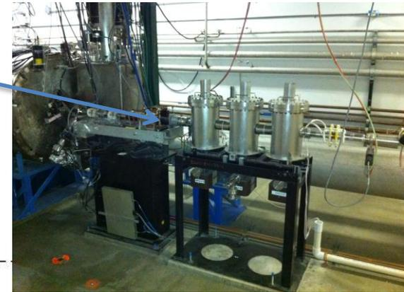
2 Superharp to measure beam profile and absolute beam position
