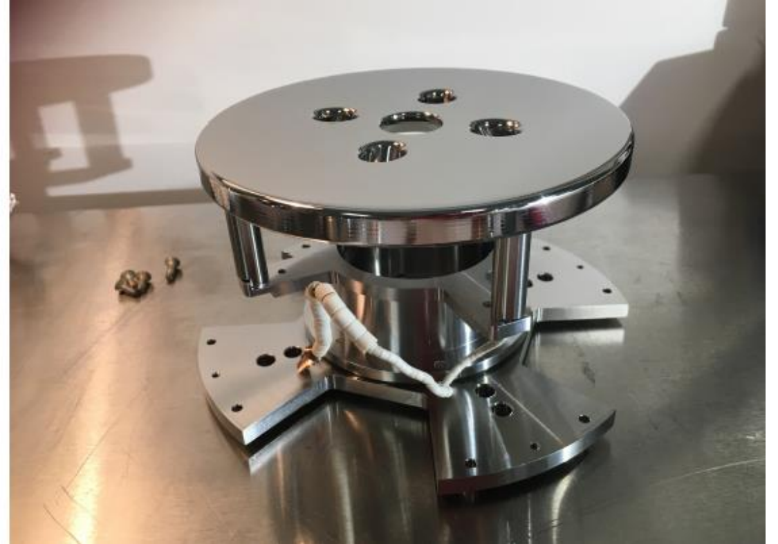
The flat anode. The anode aperture is shifted by -1.6 mm. The anode can be biased with wire visible in the photo.
