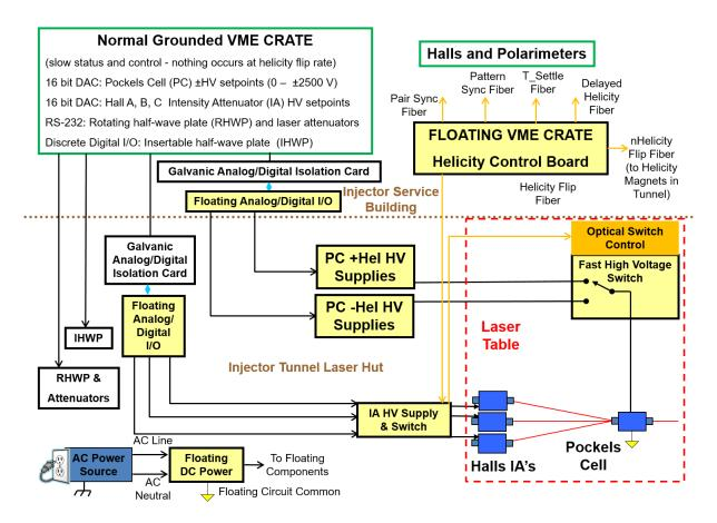
Figure 4: Electrical ground isolation.
