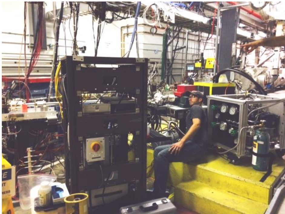
User purges bubble chamber with nitrous oxide and filling chamber.
