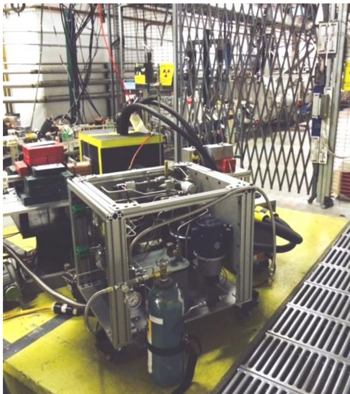
Bubble Chamber and supporting apparatus staged in the Injector Tunnel.
