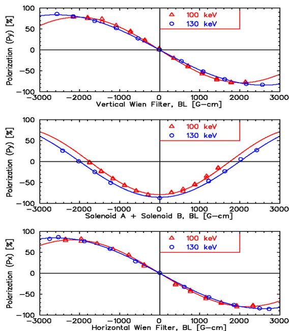
Figure 6: Variation of the electron polarization as a function of the magnetic integral for each spin rotator is shown. The two calibrations used different photocathodes, which explain the difference in maximum polarization.
