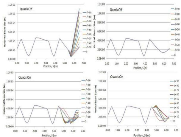
Figure 4: RMS beam size (horizontal/vertical) vs. Wien filter spin angle ( $\pm 90^\circ$  in  $10^\circ$  increments) without (upper) and with (lower) quadrupole correction.
