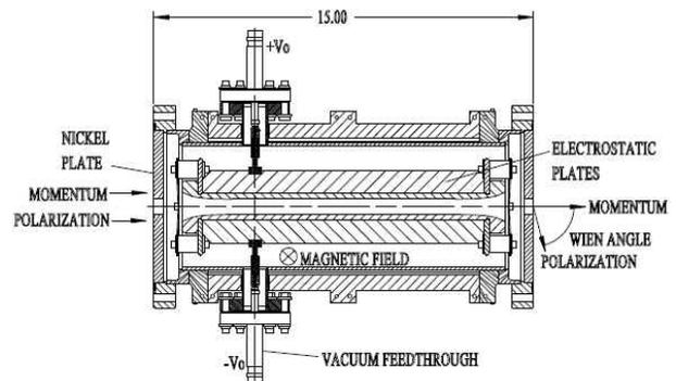
Figure 1: Diagram of Wien filter indicates the static fields and net effect on the beam in the precession plane.
