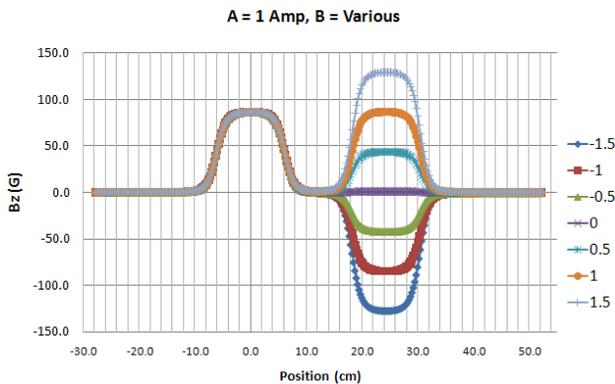
Figure 3: Measurements of the axial magnetic field for two solenoids with the first excited at 1 ampere and the second over a range of currents to add, zero or buck the net magnetic field integral (net spin rotation).
