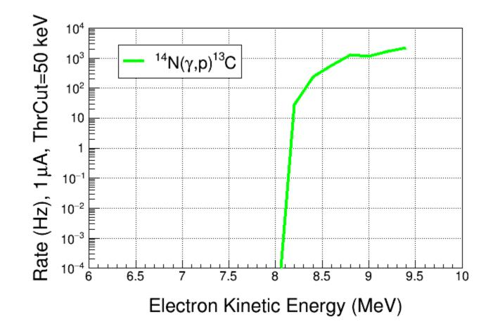
Expected rate from <sup>14</sup>N(γ,p)<sup>13</sup>C with lower operational pressure (Chamber threshold = 20 keV)
