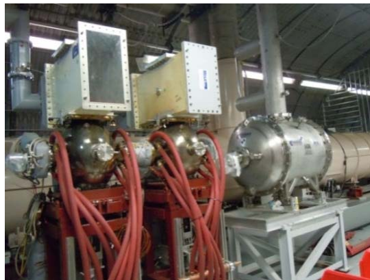
Figure 5: The 112 MHz photo-injector with 500 MHz bunching cavities inside the RHIC tunnel. The cathode stalk will be insertable from the back of the cryomodule. The cathode is illuminated by a green light from a laser (not shown in the figure). The cavity has a quarter-wave structure, with coaxial fundamental power coupler that also serves as a fine tuner.
