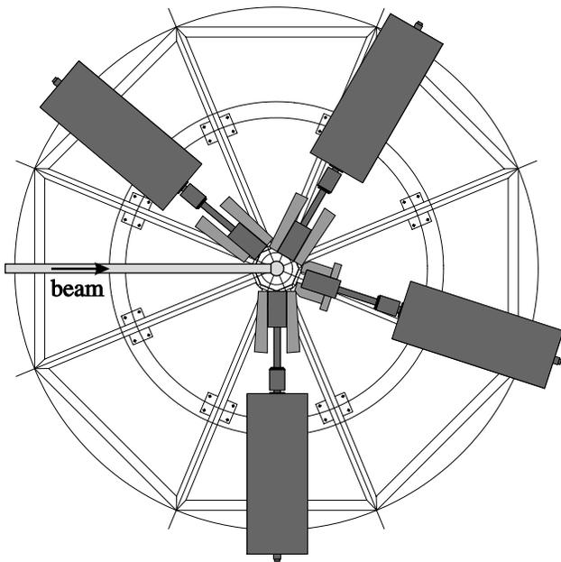
FIG. 1. Top view of the present experimental setup. The detector array used consisted of four high efficient ( $\epsilon = 100\%$ ) HPGe detectors with active BGO shielding in close geometry around the target chamber. The array was placed on a motor driven revolving table.
