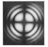
7. The dark band should be centered on the pencil mark you have placed on the screen in step 5. If it is not centered, you will adjust the pitch and yaw of the cell to move the extinction pattern. You will notice that when you manually lift the waveplate out of the beam, you will see a complete inversion of the pattern where it is in a full passing mode as seen below:
