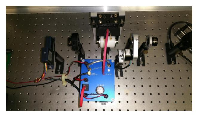
From Left to Right we see the following components: Shutter, Output LP, RTP cell, moving half wave plate, Input LP.
