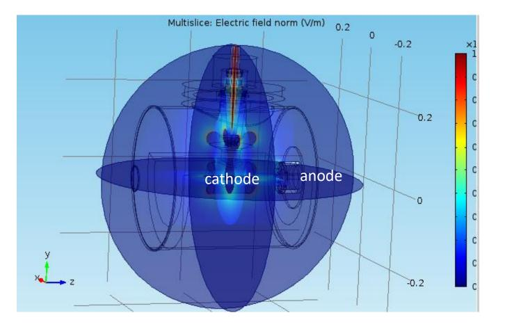
This image shows the electric field norm |E| in MV/m as color intensity. The coordinate system is as shown for all plots and images the origin is at the center of the cathode electrode. (The anode is at the right )
