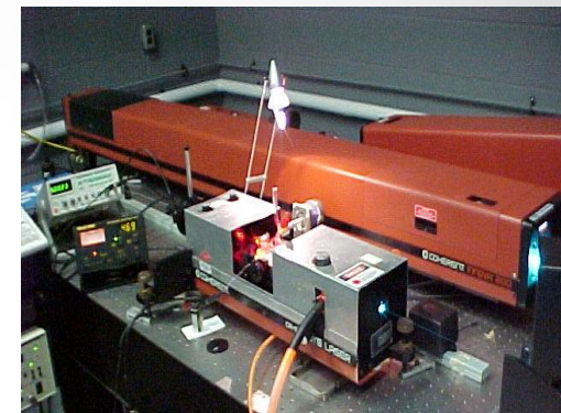
Argon ion laser (257.3 nm) frequency doubled
