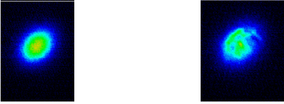
Figure 5. Beam on Be target before (left) and after (right) five minutes at 5.5 \times 10^{10} e^-/\text{bunch} train.
