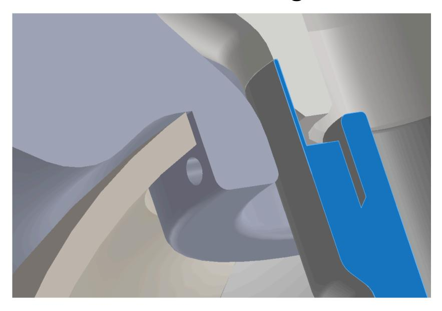
Hog out option to reduce weight, Yan's preliminary simulations show no major changes in field, but Yan will make graphs of potential along ceramic
