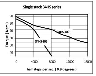
Bi-polar drive with coils in parallel
