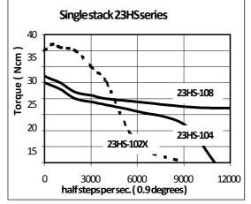
Bi-polar drive with coils in parallel
