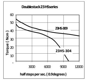
Bi-polar drive with coils in parallel
