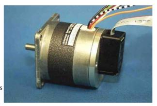
Where customers require an encoder for use with control systems not supplied by Mclennan and which require alternative line-counts, the model 'RI' encoder is available with any line count required up to a maximum value of 2,000 ppr. resulting in a measuring resolution of 8,000 steps/rev.
