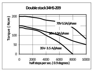
Bi-polar drive with coils in parallel
