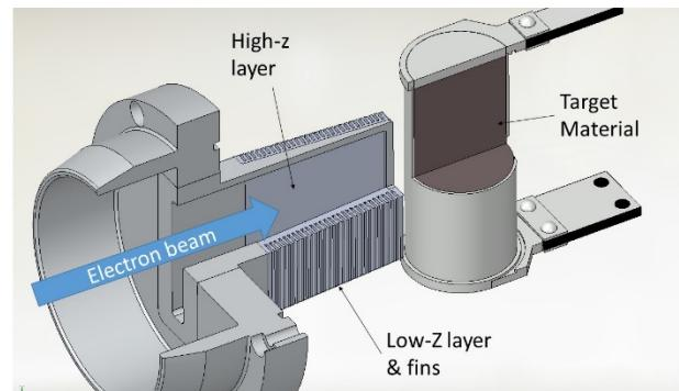
Figure 1: Layout of the converter and photofission target.
