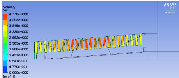
Figure 3: Cross-section through the horizontal plane along the beam axis showing flow balance in water between all fins.
