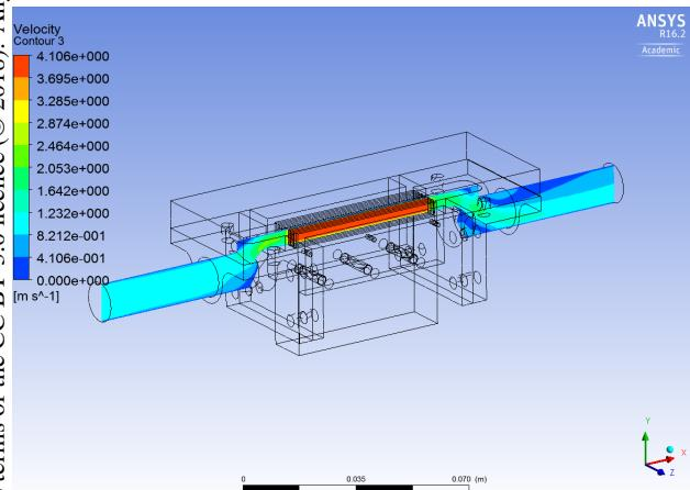
Figure 7: ANSYS CFX Converter Prototype showing flow velocity through the vertical mid plane.
