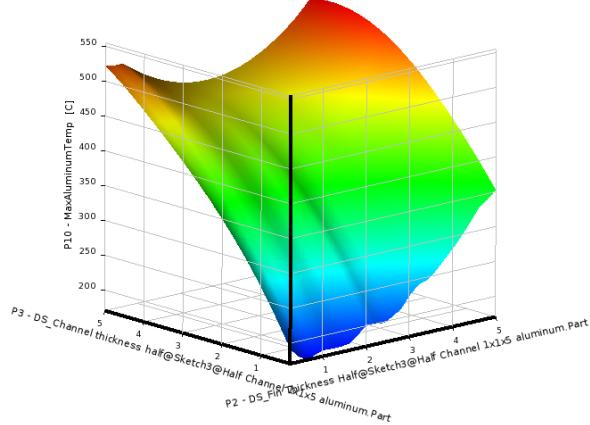
Figure 4: Response Surface of fin optimization showing temperature as a function of fin thickness and channel thickness.
