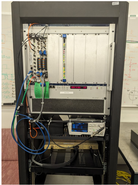
Figure 1. SEE BPM rack, assembled for testing M15 and stripline BPM sensors.
