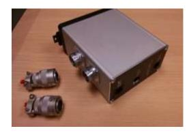
The laser shutter we are presently using is the LST400. This shutter has TTL logic feedback of shutter position, which is less than ideal for our safety systems feedback, so we have placed relays on our board that are opened and closed based on the state of the TTL signal. This provides dry contact information more suitable for feedback. There is one relay for the open state indication, and another for the closed state.
