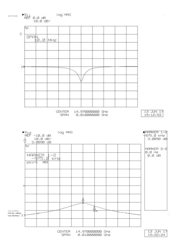
The cavity has a measured Q of 7,677. Because the coupler is matched, the unloaded  $Q_0$  is twice this or 15,334.
