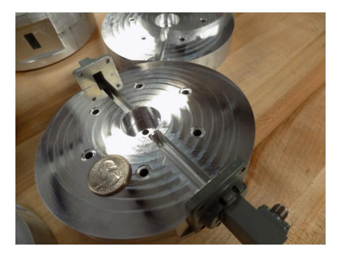
The cavities were constructed in two halves and bolted together. The waveguide is WR-62 (that is .62 inches wide) and spans the frequency range of 12-18 GHz. The bore is 5mm.
