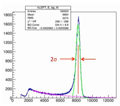
After time-of-flight cuts, the Gaussian fit (green) is made after the exponential quasi-inelastic tail is temporarily subtracted.
