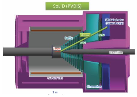
SOLID/PV-DIS: e<sup>-</sup> - <sup>2</sup>H: Statistical polarization accuracy required ~0.5%
