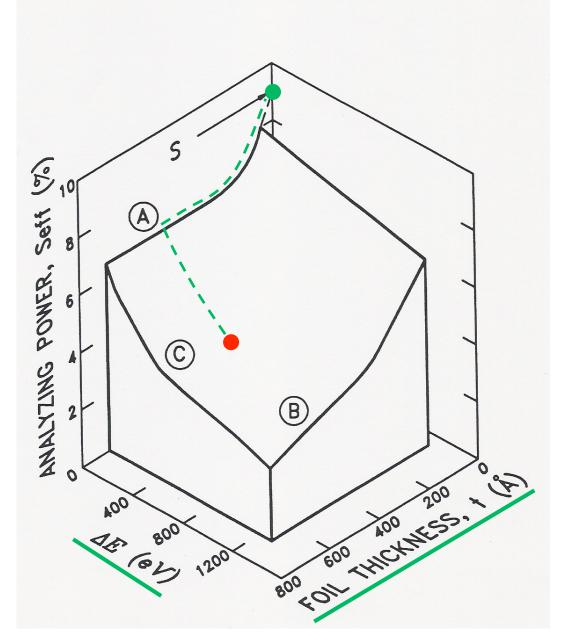
The Sherman function is calculated assuming elastic scattering from single atoms. However, the higher the incident energy, the flatter this landscape becomes. This, and the ease with which TOF corrections can be made, are the major advantages that making measurements at 5 MeV (as opposed to, e.g., 120 keV) give us.
