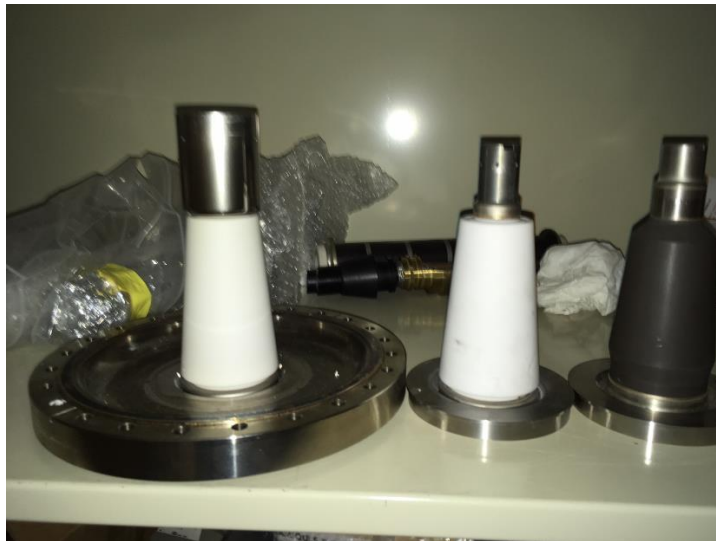
4 One of the white R28s welded to a hogged out 10" flange
