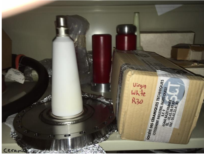
3 The only remaining white R30 already welded to 10" flange
