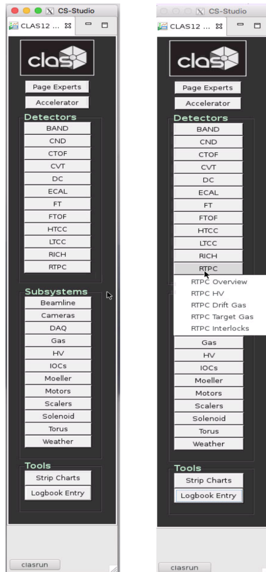
Figure 5: CS-Studio for the slow controls of the CLAS12 (left: general, right: RTPC options)
