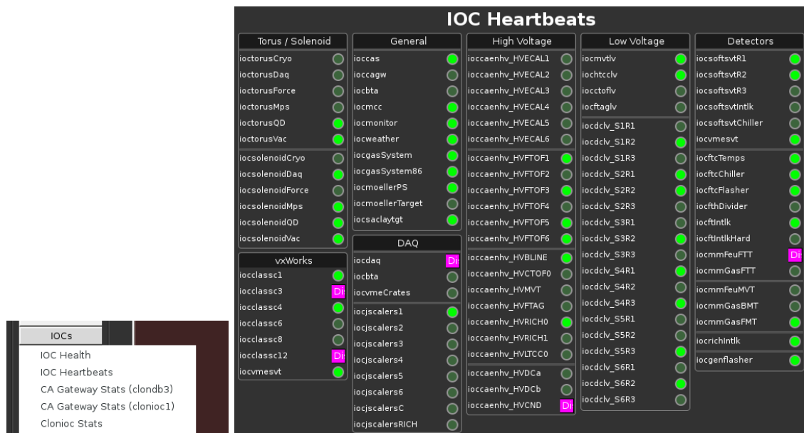
FIG. 5: Dropdown menu (left) from the IOCs button in the main CLAS12 controls menu showing links to the IOC health and heartbeat screens (right). The static pink “Disconnected” heartbeats here are IOCs that are intentionally offline at the time of this screenshot.
