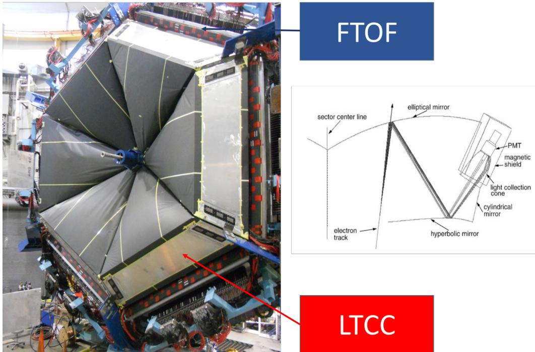
Figure 1: Left: The LTCC sectors installed on the Forward Carriage. The Forward Carriage is roughly 10 m in diameter. Right: The path of Cherenkov photons to the PMTs.
