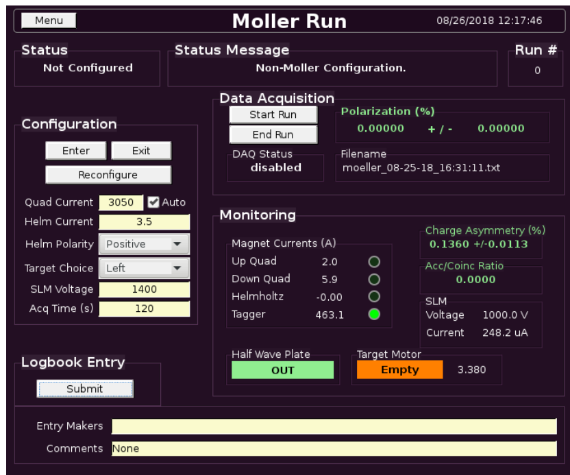
FIG. 1: The user interface for shift workers for operating a Møller run is divided into Status , Configuration , Data Acquisition , Monitoring , and Logbook sections. In this screenshot, the Møller system is not configured, according to the Status section, i.e. the setup is for non-Møller beam delivery.
