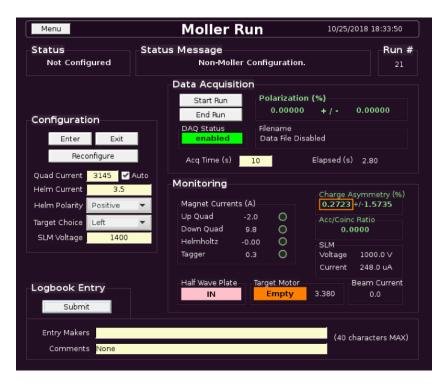
FIG. 1: The user interface for shift workers for operating a Møller run is divided into *Status*, *Configuration*, *Data Acquisition*, *Monitoring*, and *Logbook* sections. In this screenshot, the Møller system is not configured, according to the *Status* section, i.e. the setup is for non-Møller beam delivery.
