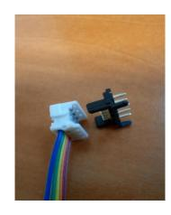
4) Disconnect the fiber side interface PCB (easier than side Pmt block)
