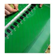
5) Exchange the PMt block and its fiber and inverse this procedure for mounting
