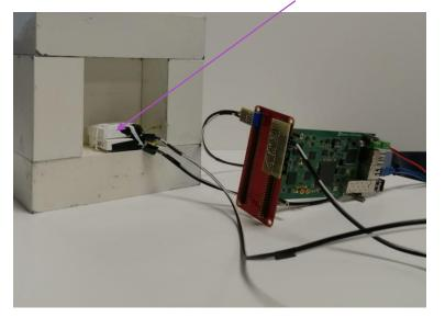
Two channel coincidence (implemented at firmware level) used as trigger for PHA acquisition
