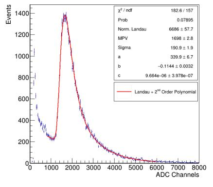
Pulse Height Cosmic Rays - 2-Channel Coincidence
