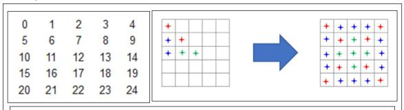
Left: Typical crystal labeling as the beam sees them; Right: possible positioning of the 2 SiPM channels. The nominal positioning will be the central crystal and one location on the cross (green symbols)
