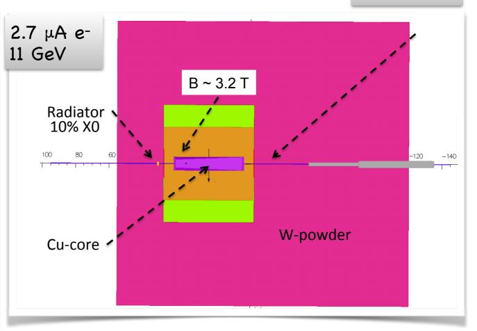
$1 \times 10^{12} \gamma/s$  - more that 30 times that of 100 na mixed electron photon beam
