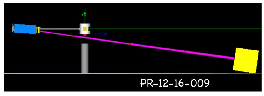
While these both moved the dump away from the pivot they suffered from the 'sheet of flame' – the dispersion of the beam after the dipole due to bremsstrahlung and multiple scattering in the radiator
