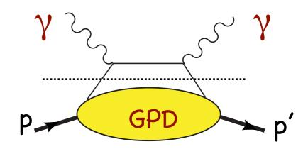
Provided that s, t, u >>  $\Lambda^2$  the handbag mechanism involves factorization of the amplitudes into:
