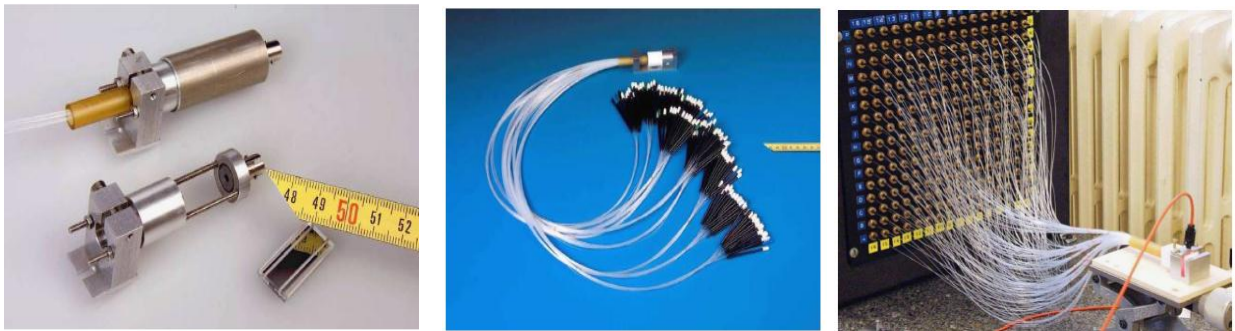
Fig. Some details of CMS calorimeter laser based monitoring system (adopted from M. Anfreville et al., NIM A 594, 2008, p292)
