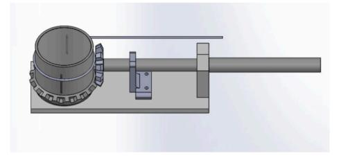
The rotating target cup driven by a gear and shaft with the NMR loop
