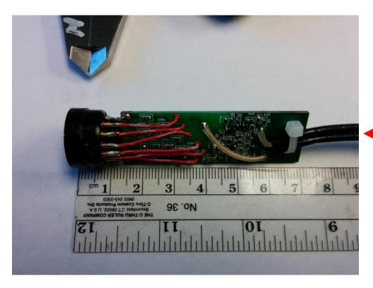
HyCAL readout is on top, through printed board strips that each are slightly movable to get access to PMTs and dividers (unscrew on top to move a bit laterally, on bottom can just push a bit).
