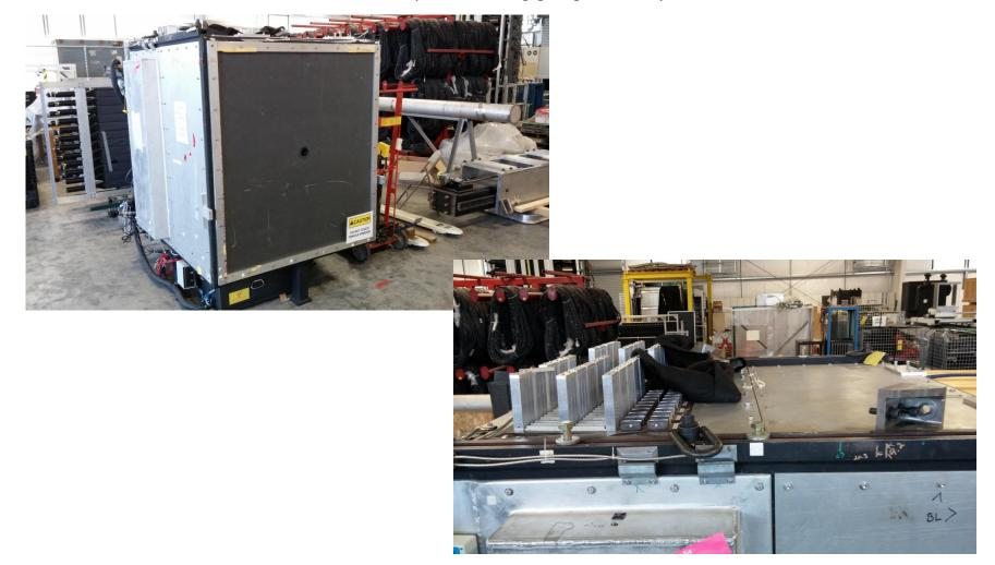
HyCAL readout is on top, through printed board strips that each are slightly movable (unscrew on top to move a bit laterally, on bottom can just push a bit).
