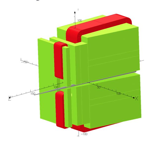
Iron weight is of 15 tons Coils weight is of 1.5 tons
