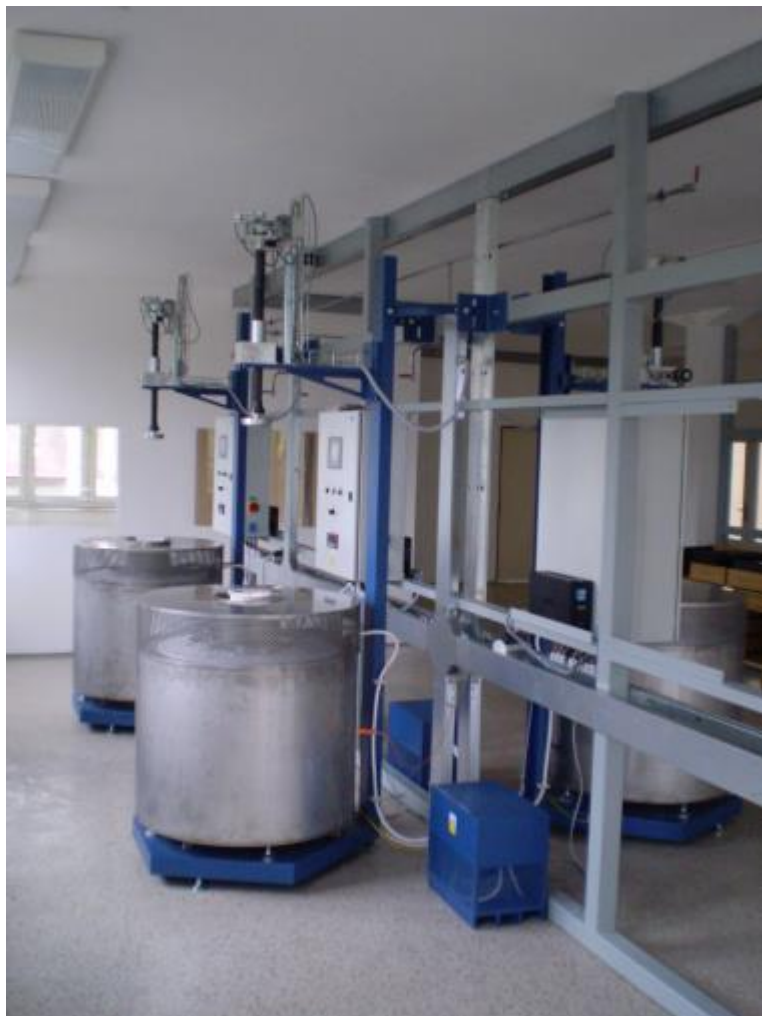
Picture no.3: Crystal growth furnaces in new premises
