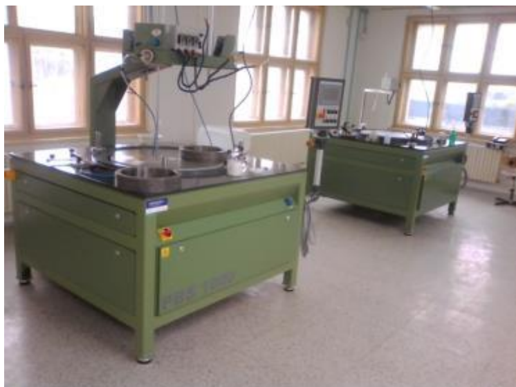
Picture no. 4: Lapping and polishing machines
