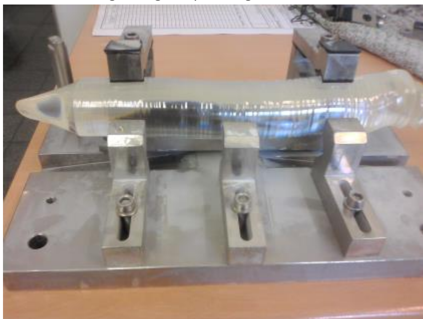
Picture no. 2: Holder for cutting of crystals
