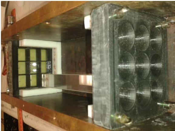
Fig. 17. (color online) Neutral Particle Spectrometer (NPS) prototype produced with 3D printing technology.
