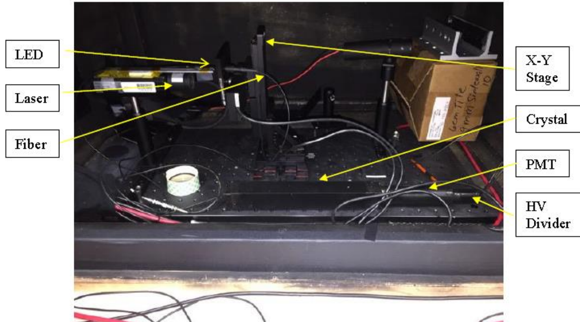
Fig.1 The NPS/COMCAL readout test setup
