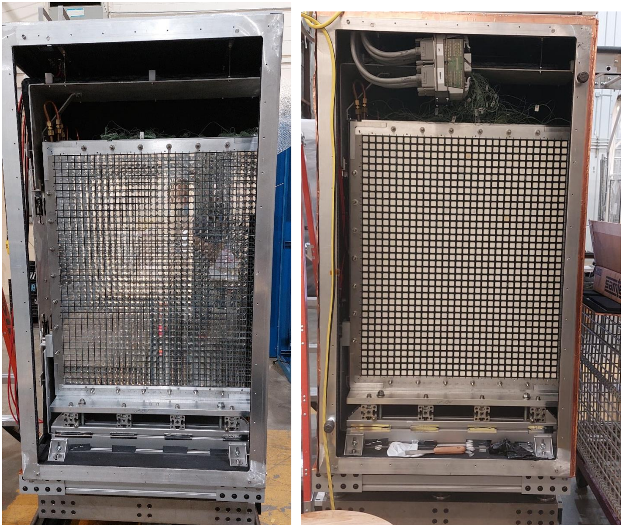
Fig 1: View of the detector front face. The left picture shows the bare crystals and the right picture shows them covered by reflective material glued to plastic covers. Each crystal can be uncovered individually by removing its corresponding cover (see Fig.4).
