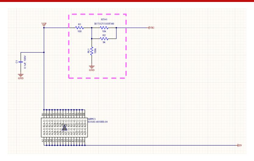
Assumed Root Cause: Corner frequency caused by high impedance in the temperature correction circuit
