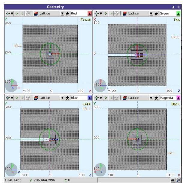
Concrete shielding box: 2m x 2m x 2m, with entrance tunnel
