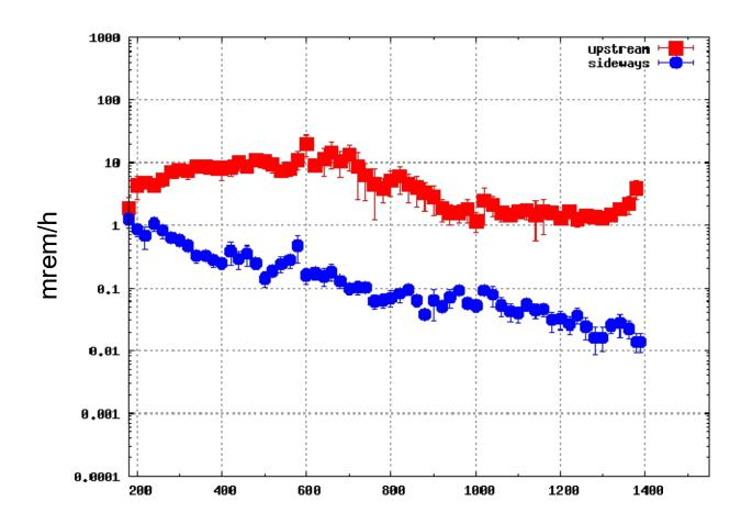
Upstream means 20 < R < 50, NOT include the beam pipe, sliding door not shift to park mode yet!
