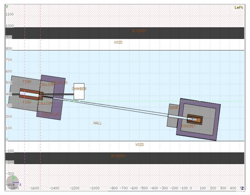
40 cm collimator box + 100cm tungsten pipe Collimator shielding: 100cm concrete + 100 cm borated plastic
