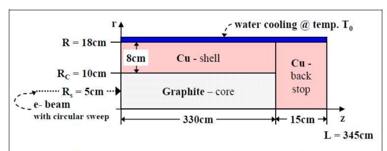
Figure 16: Baseline design of the 25GeV / 300kW main dump for the XFEL with slow (not intra train) beam sweep of  $R_s = 5$ cm and  $\sigma_{beam} \ge 2$ mm.
