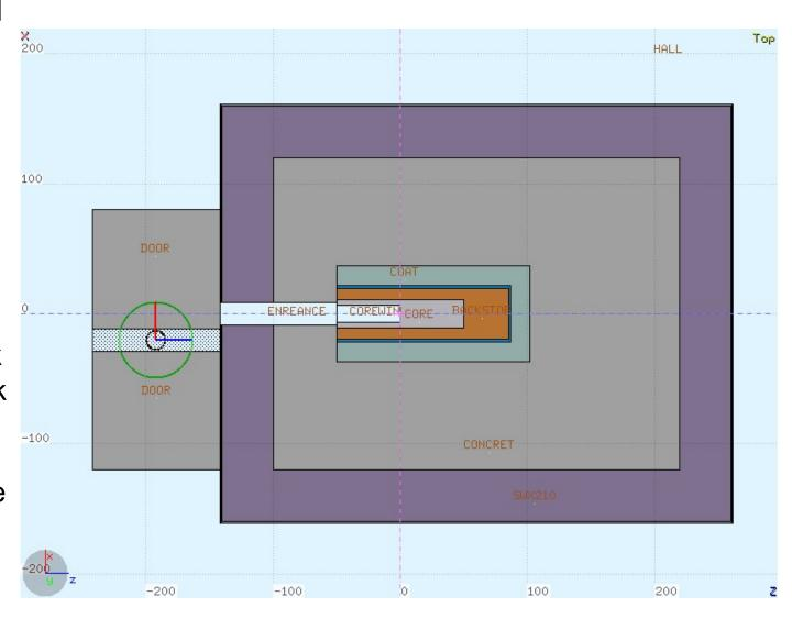
Shift the door to its horizontally right by 20cm when the beam is off to block the dump entrance
