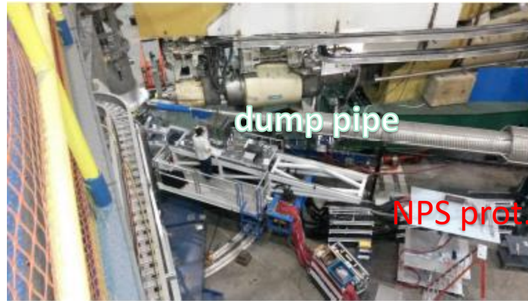
The NPS Prototype installation in Hall A. From left to right the scattering chamber, beam line, the DVCS calorimeter and the stand with Prototype can be seen.
