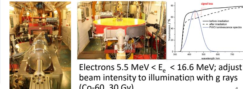
Electrons  $5.5 \text{ MeV} < E_e < 16.6 \text{ MeV}$ ; adjust beam intensity to illumination with g rays (Co-60, 30 Gy)
