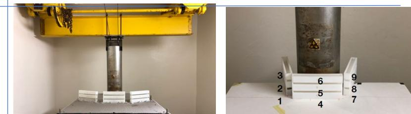
Co-60 source, 222 TBq, simultaneous irradiation of nine crystals/water; different dose rates possible
