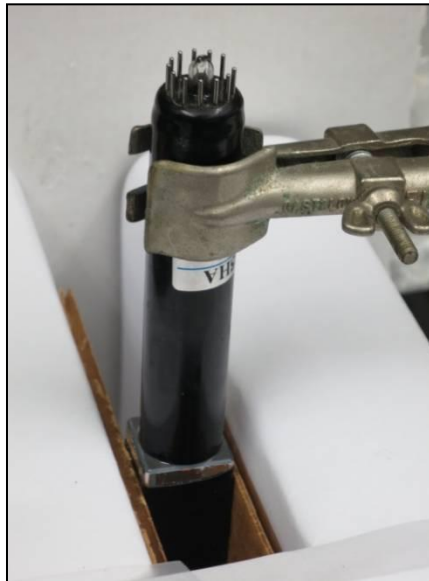
Attaching PMT with optical glue
