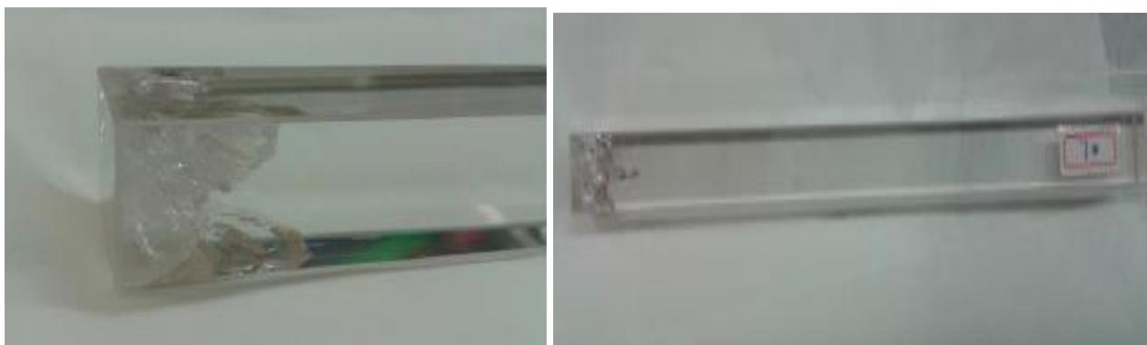
Fig.8: Block #1 damage due to irradiation at dose rate  $\sim 13$  Mrad/h. Rapid and not uniform rise temperature cracked the crystal sooner than we could stop the beam.
