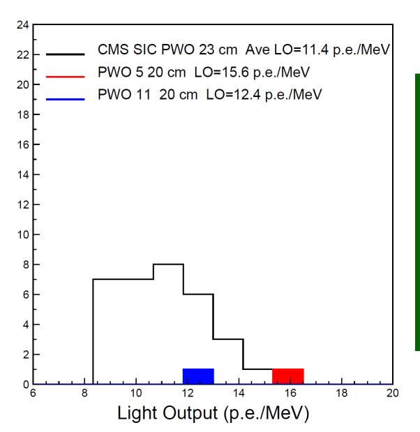
Light output of both samples are larger than the average of **CMS PWO** crystals as published in IEEE Trans. Nucl. Sci. NS-51 1777.
