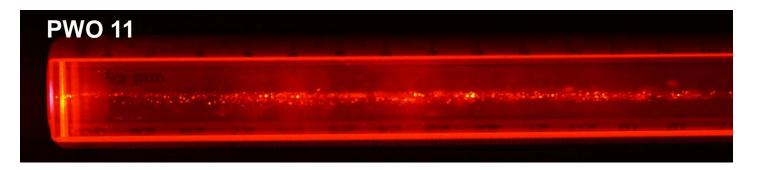
Sample 11 has significant scattering centers in the bulk
