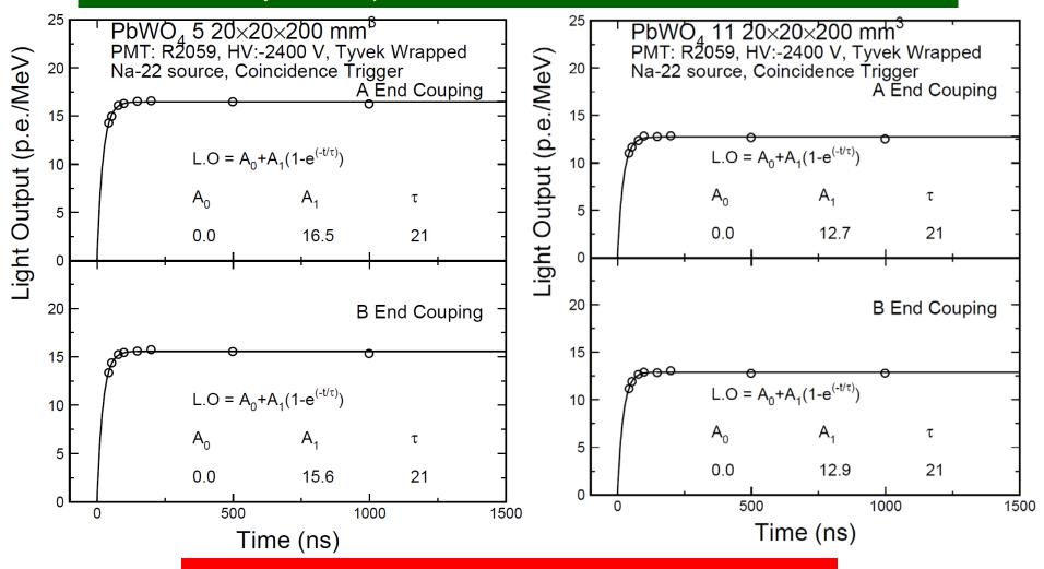
Both samples are faster than CMS PWO crystals
